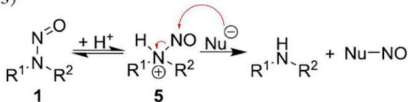
Scheme 2. Proposed Mechanism for Nitrosamine Denitrosation in Acid via the N-Protonated Conjugate Acid (5)
