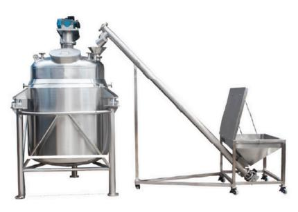
This tank is designed for the manufacturing of Sugar & Liquid Glucose syrup. It comes with a drive motor anchor agitator system to manufacture consistent & high-quality syrup. Its steam jacketed arrangement, along with third layer rock wool insulation & SS Cladding to conserve temperature.
