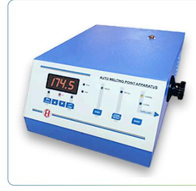
The 'Start' switch is used to start the measurement of melting point. User can stop the process of measurement using 'Stop' switch after the instrument reaches the melting point of the sample. The display will always show the last temperature where 'Stop' switch was pressed in last.
