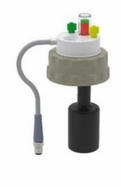
To prevent your waste canister from overflowing, connect these <u>b.safe</u> waste caps with electronic fill-level control to the alarm box. When the 'canister full' level is reached, you will receive an optical and acoustic warning. The alarm is triggered before your canister is completely full. This leaves a small safety buffer in the canister.
