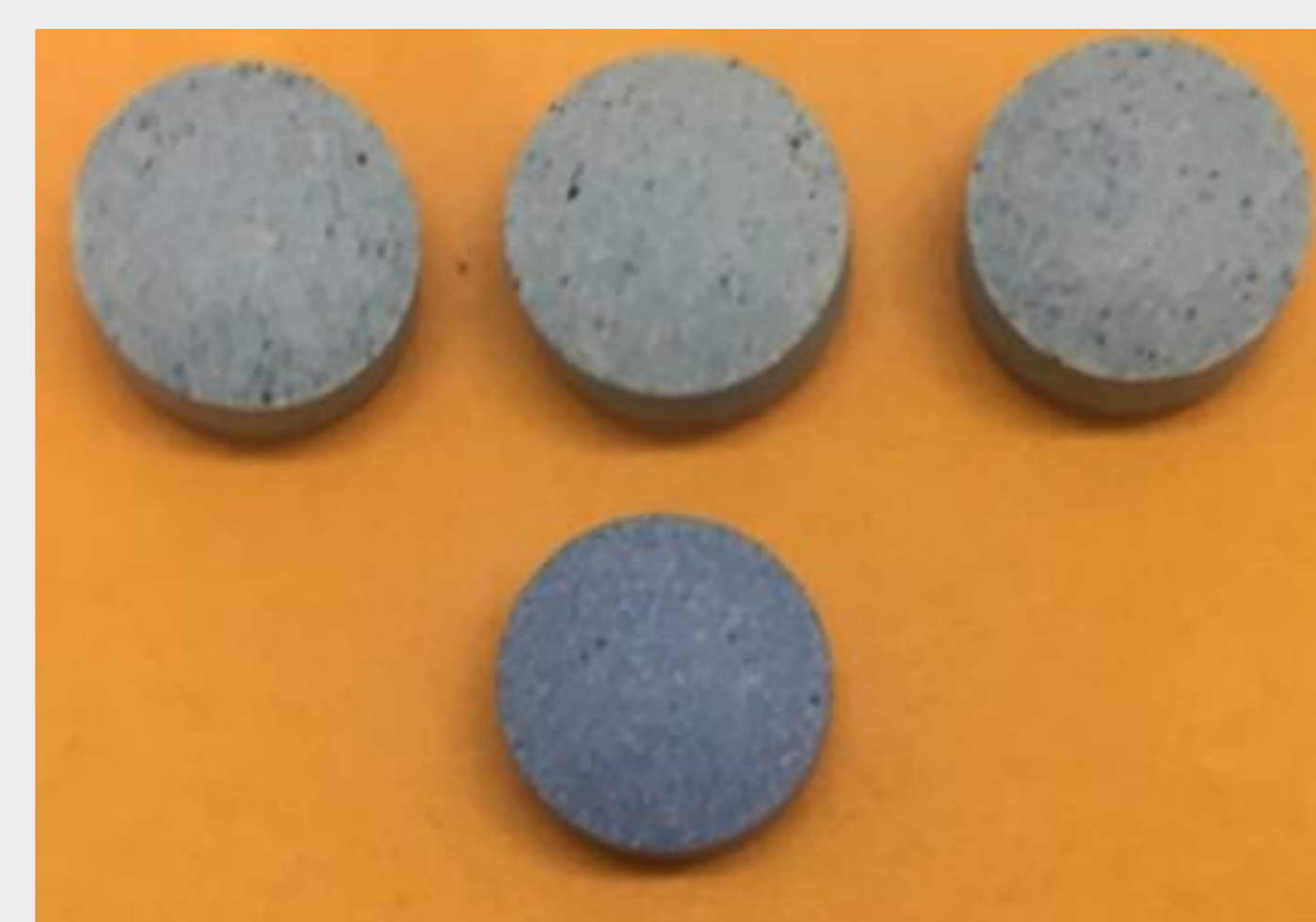
Figure 1. Tablets stressed at 80°C/73% RH/1 day, representing \Delta E^*=9.3 (top) vs. control tablet (bottom).
