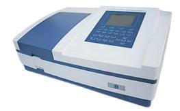
Double Beam Spectrophotometer is a solid state microprocessor based instrument designed for quick and accurate spectrophotometric analysis of any concentration. It operates at a wavelength range of 190 nm to 1100 nm. The use of diffraction grating in the monochromator produces a linear spectrum. The grating having very high resolution of 1200 lines/mm ensures a narrow bandwidth.
