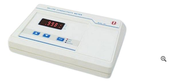
Digital Conductivity Meters are reliable and accurate test instruments for measurement of Conductivity of aqueous solutions. They measure Conductivity and TDS in five ranges. The Resolution is 0.1 µS/cm and 0.1 ppm respectively, in the lowest range. The cell constant is flashed on a digital display & can be adjusted from the front panel..
