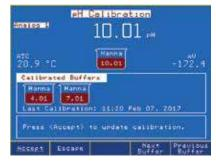
Up to five-point pH calibration with automatic buffer recognition
